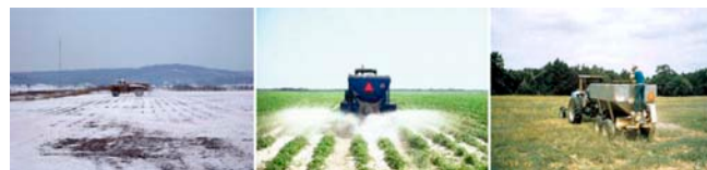
Figure 4-1. FGD gypsum can be applied directly to the soil surface using conventional dry material spreaders. (From the FGD Network website: http://www.oardc.ohio-state.edu/agriculturalfgdnetwork .)
